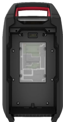
Figure 1-11 : Connexion satellite non installée
