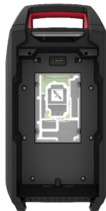
Figure 1-12: Satellite Connection Installed
